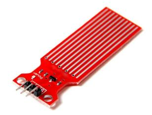
Water sensor is designed for water detection, which can be widely used in sensing water level. Connecting a water sensor to an Arduino is a great way to detect a water molecule.
