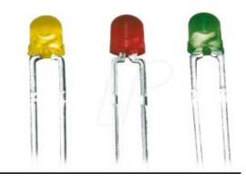
A light-emitting diode (LED) is a semiconductor light source that emits light when current flows through it. Electrons in the semiconductor recombine with electron holes, releasing energy in the form of photons. The color of the light (corresponding to the energy of the photons) is determined by the energy required for electrons to cross the band gap of the semiconductor. White light is obtained by using multiple semiconductors or a layer of light-emitting phosphor on the semiconductor device.
