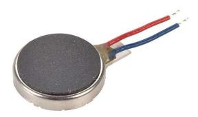
Vibration motor is a DC motor in a compact size that is used to inform the users by vibrating on receiving signals grove - Vibration Motor consists of one-coin type motor which is a permanent magnet coreless DC motor. It vibrates when the input logic is high which can be used to notify the user. Integrated with Grove interface, it provides a simple way to connect with Arduino boards without soldering.
